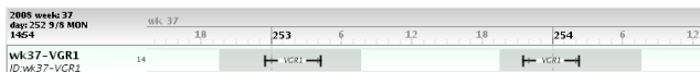
Figure 4. An example of a request reference violation: though both tracks fall within their viewperiods, the required separation interval between the tracks must be at least 24 hours. In this example the tracks are separated by approximately 12 hours.
